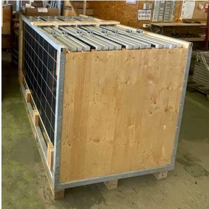
Figure 2: Transport box for four SSB4 units
