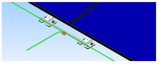
Additional continuous north-south wires must be installed within the generator at the prescribed distance (every 5m, 10m or 15m depending on the lightning protection class) and connected to all module carriers:
