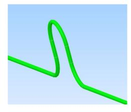
The north-south wire can be easily pulled through using an expansion loop at the thermal separation line.
