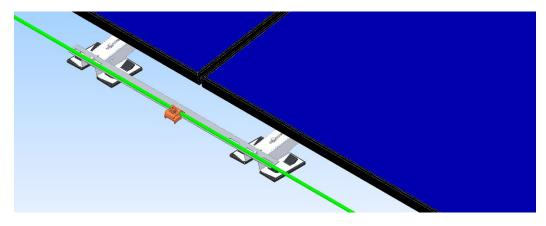
Otherwise, the connection is made directly to the foot of the module carrier:
