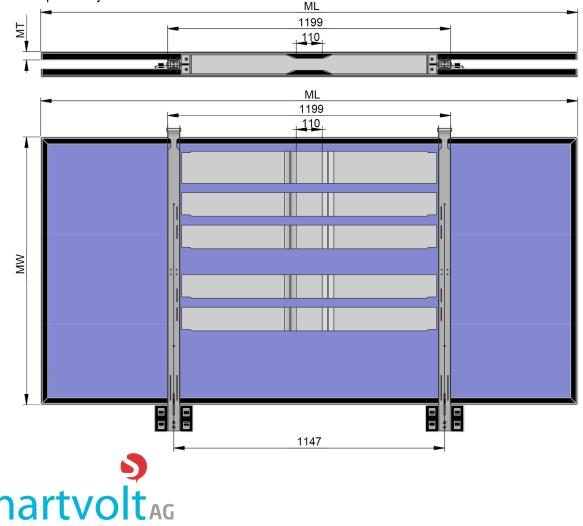
There are no restrictions in the space outside the 1199mm area. Within this area only in the center 110mm is enough room to situate the junction boxes. The free space below the junction box Therefore, be 6mm minimum.
