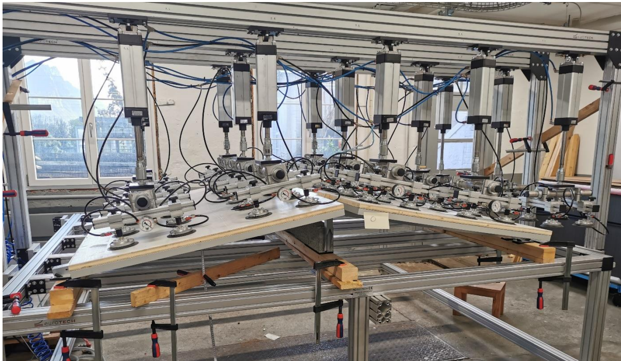
Illustration 1 Test setup for snow load testing of the SmartSolarBox Version 5.0
