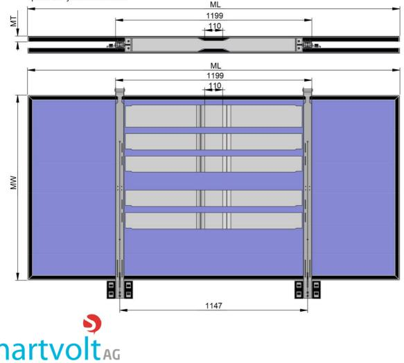
There are no restrictions in the space outside the 1199mm area. Within this area only in the center 110mm is enough room to situate the junction boxes. The free space below the junction box has to be 6mm minimum.
